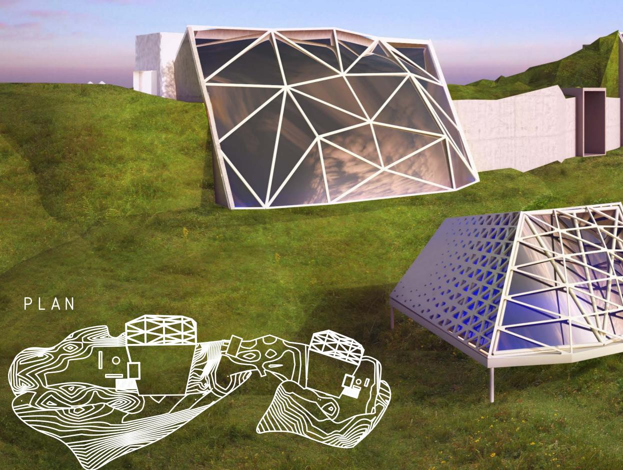
USING THE LANDSCAPE AND ENVIRONMENT TO THE MAXIMUM ADVANTAGE, OUR PROJECT USES THE TERRAIN AND ITS FEATURES AS THE DRIVING FORCE OF THE DESIGN.BURYING THE PROGRAM IN THE GROUND AND ADDING CENTRAL CHIMNEYS ALLOWS FOR REGULATION OF TEMPERATURE TO AVOID DEPENDANCE ON ELECTRICITY FOR HEAT.ADDITIONALLY THE PARAMETRICALLY DESIGNED WINDOW FACADE TILTS BACKWARDS TO ALLOW FOR A GREATER VIEW OF THE SKY.
