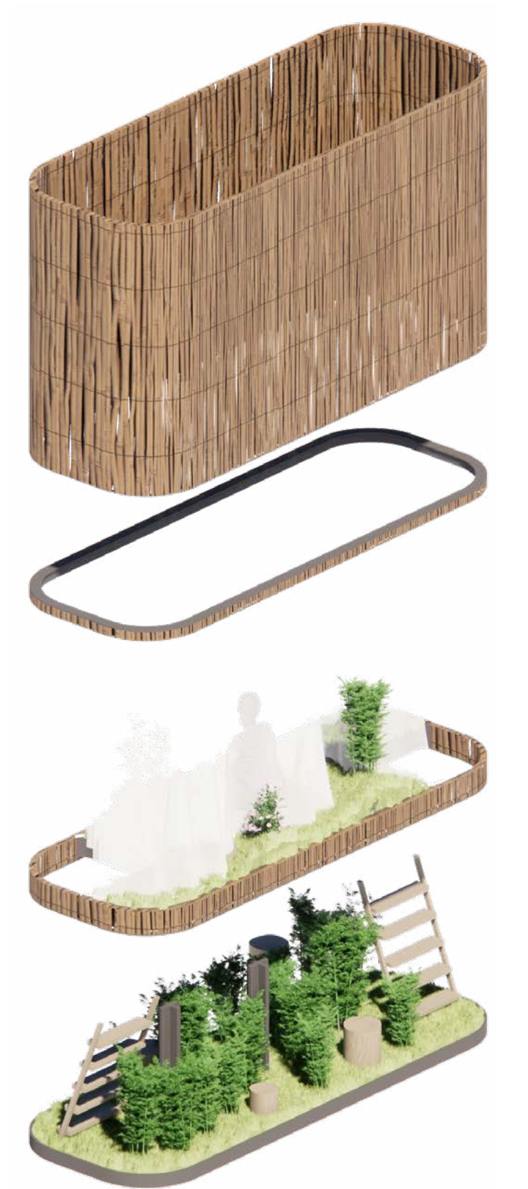
Exploded Axonometric showing simple assembly layers
